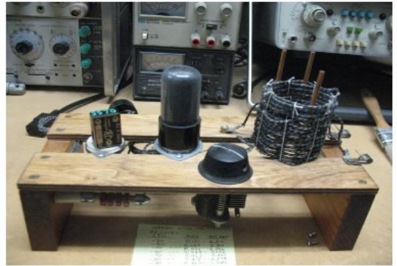
Years later Jim built this replica of his first cw transmitter, as described in the 1950 ARRL Handbook [Willie Baber, WJ9B, photo]
