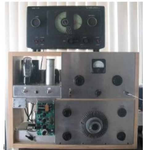
Hallicrafter s-38 and homebrew 1950s technology; 83 rectifier, 6v6 oscillator, and 3 tube regen receiver, plus a modern audio filter [Willie Baber, WJ9B, photo]
